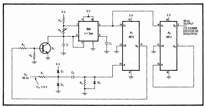
On time. Three-chip multiplier converts 50-Hz power-line frequency into 60 Hz for devices used in the U. S. A<sub>1</sub> generates six pulses for every 50-Hz cycle, forcing 555 timer to generate average frequency of 300 Hz. A<sub>2</sub> provides divide-by-five function on 555 waveform.
